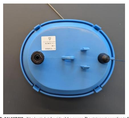
Label with **FCC ID: 2ALN6DOM** will be located at the side of the sensor. The statement according to FCC part 15 §15.19(a)(3) is placed in User's Manual, page 12.
