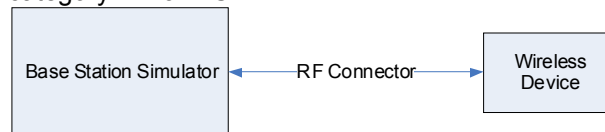
Figure 9-2 Power Measurement Setup
