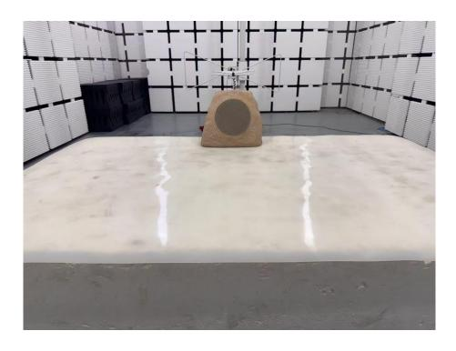
Set-up for Radiated Spurious Emission, Above 1GHz
