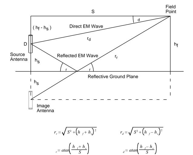
**Figure 1. UT MPE Calculation Geometry**
