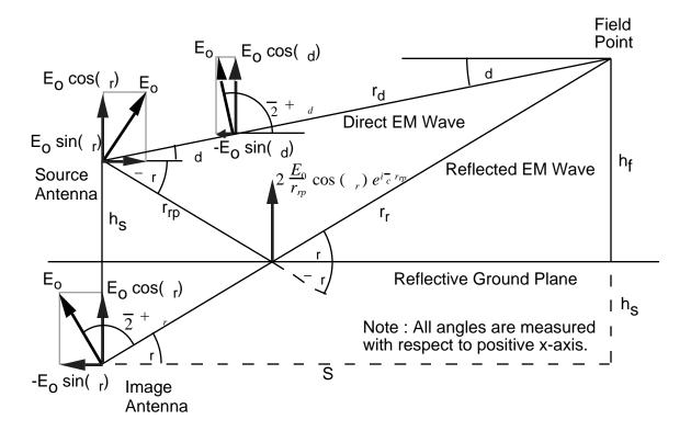
Distance to Ground Plane Reflection Point  $r_{rp} = h_s \csc(r)$
