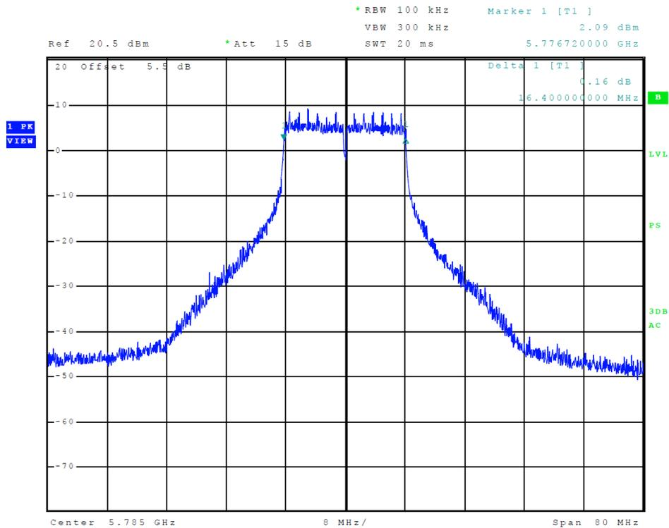
**Figure 20 Plot of Transmitter Emissions (5725-5850 MHz Band, 802.11a, 6-dB OBW)**
