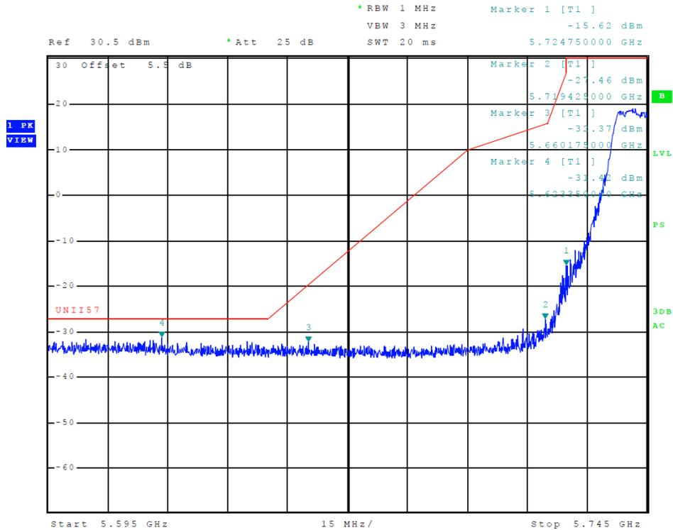
Figure 15 Plot of Transmitter Low Band Edge (5725-5850 MHz Band, 802.11a)
