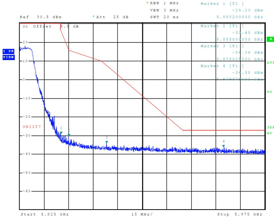
Figure 17 Plot of Transmitter High Band Edge (5725-5850 MHz Band, 802.11a)
