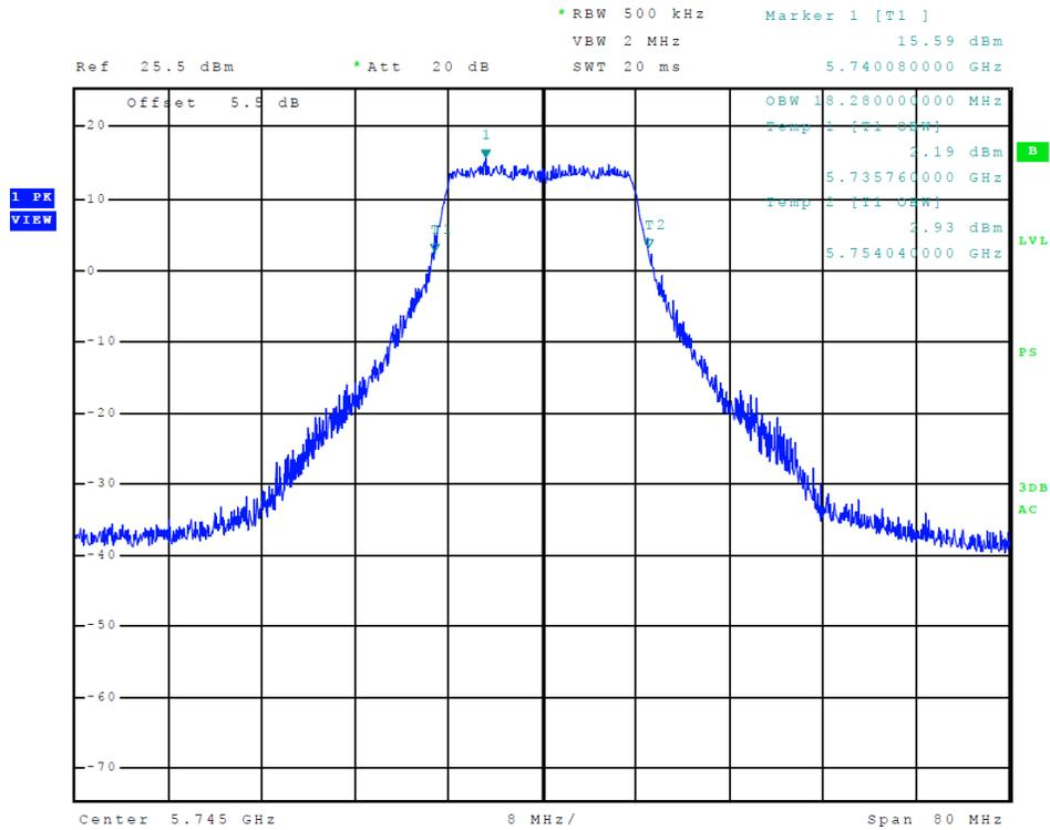
**Figure 19 Plot of Transmitter Emissions (5725-5850 MHz Band, 802.11a, 99% OBW)**
