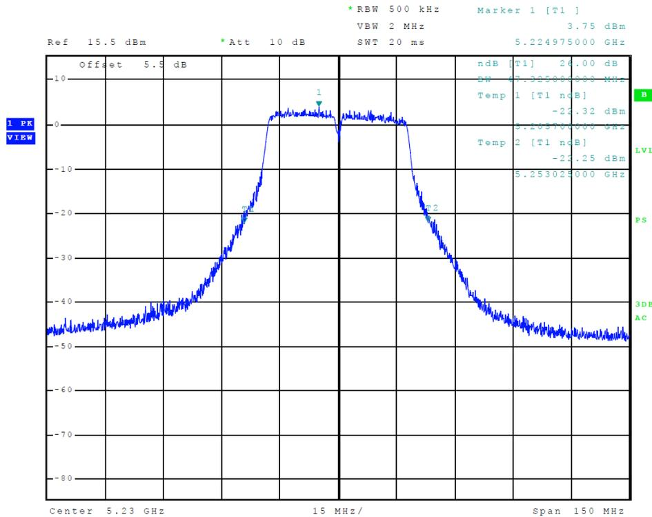
Figure 12 Plot of Transmitter Emissions (5150-5250 MHz Band, 802.11n40, 26 dB OBW)
