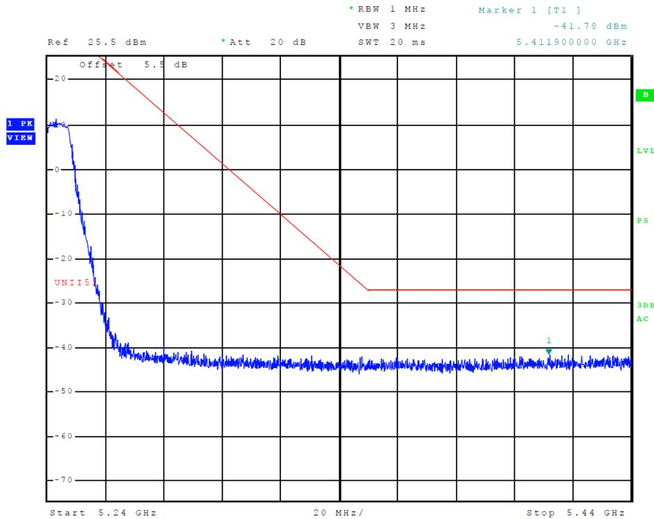
**Figure 7 Plot of Transmitter High Band Edge (5150-5250 MHz Band, 802.11a)**
