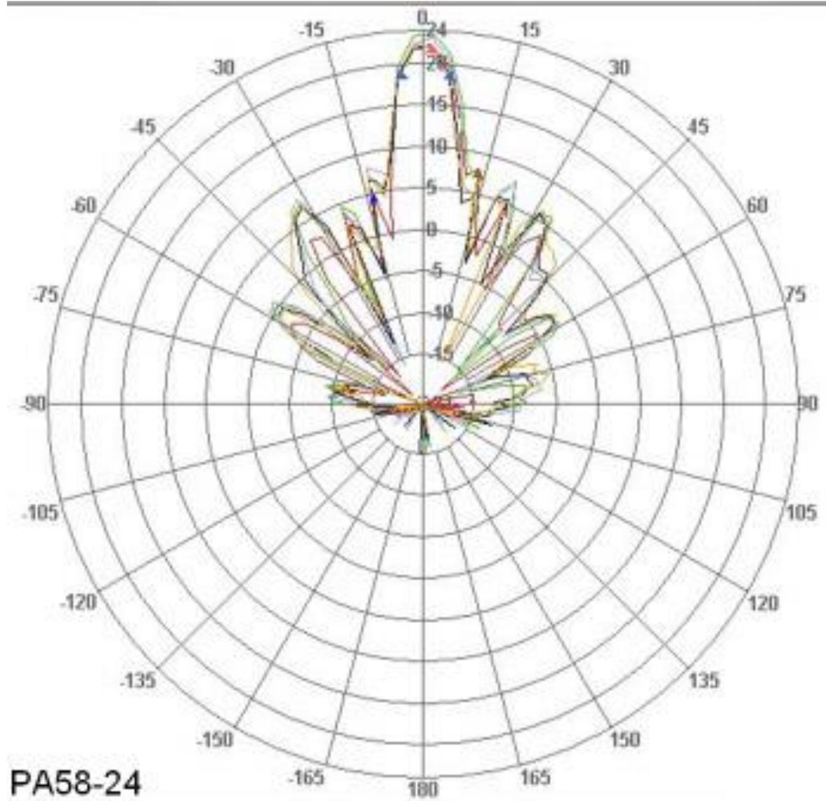
**Elevation Compliance Dish Antenna (32 dBi) HDDA5W-32-DP2**
