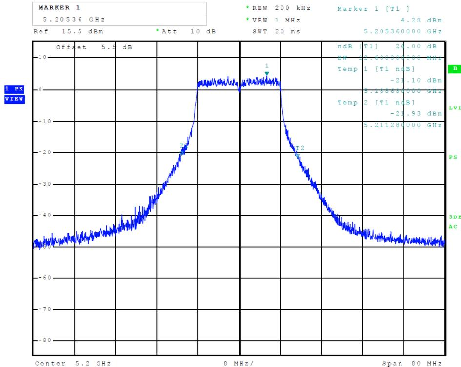
Figure 10 Plot of Transmitter Emissions (5150-5250 MHz Band, 802.11a, 26 dB OBW)
