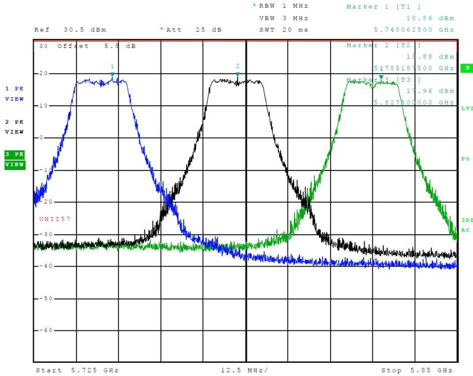
Figure 13 Plot of Transmitter Emissions (Across 5725-5850 MHz Band, 802.11a)
