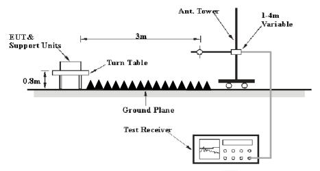
The radiated emission tests were performed in the 3 meters chamber test site, using the setup accordance with the ANSI C63.4-2009. The specification used was the FCC 15.209, and FCC 15.247 limits. The external I/O cables were draped along the test table and formed a bundle 30 to 40 cm long in the middle.
