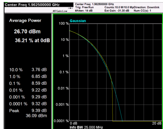
Channel: MIDDLE, Modulation: 64QAM, BW=20MHz, CCDF
