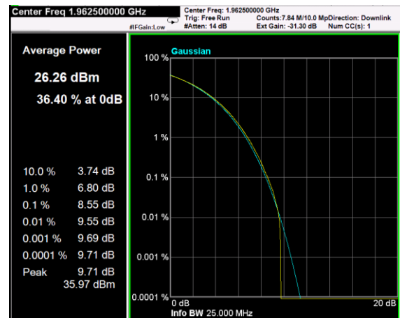
Channel: MIDDLE, Modulation: 16QAM, BW=15MHz, CCDF
