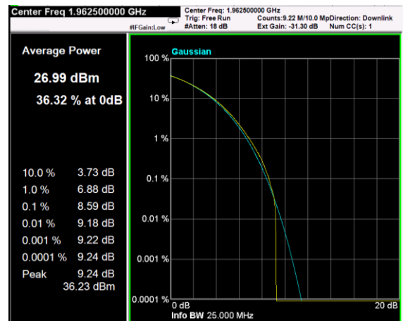
Channel: MIDDLE, Modulation: 64QAM, BW=10MHz, CCDF
