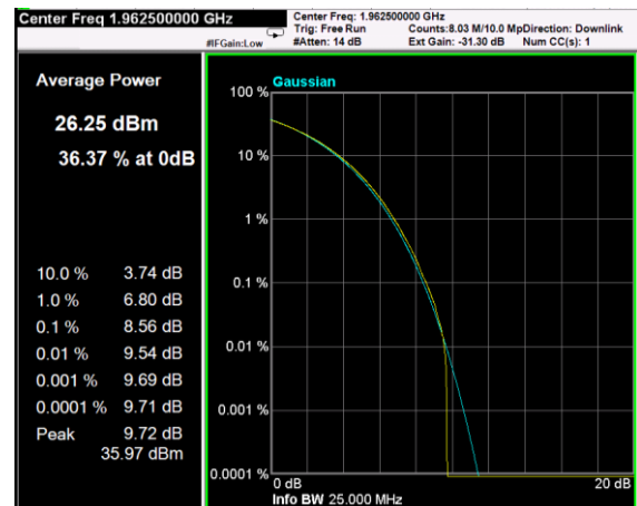
Channel: MIDDLE, Modulation: 256QAM, BW=15MHz, CCDF
