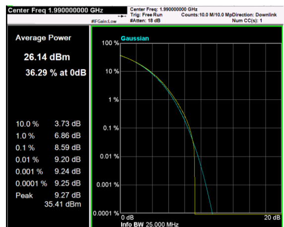
Channel: TOP, Modulation: 64QAM, BW=10MHz, CCDF
