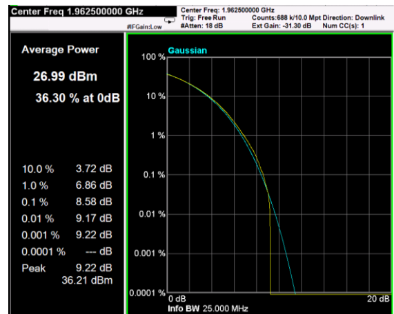
Channel: MIDDLE, Modulation: 256QAM, BW=10MHz, CCDF
