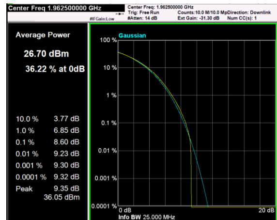
Channel: MIDDLE, Modulation: 256QAM, BW=20MHz, CCDF
