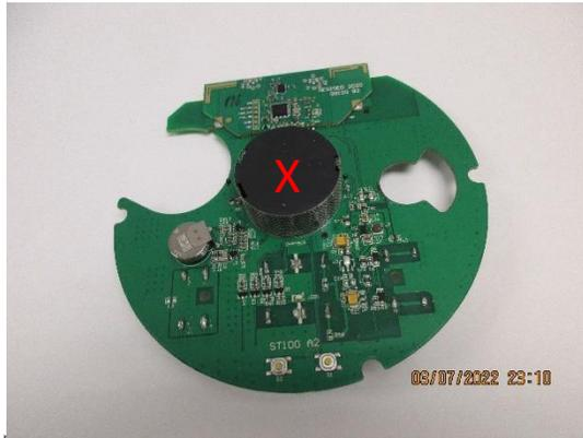
Figure 5 SIXCOMBOV with smoke chamber
