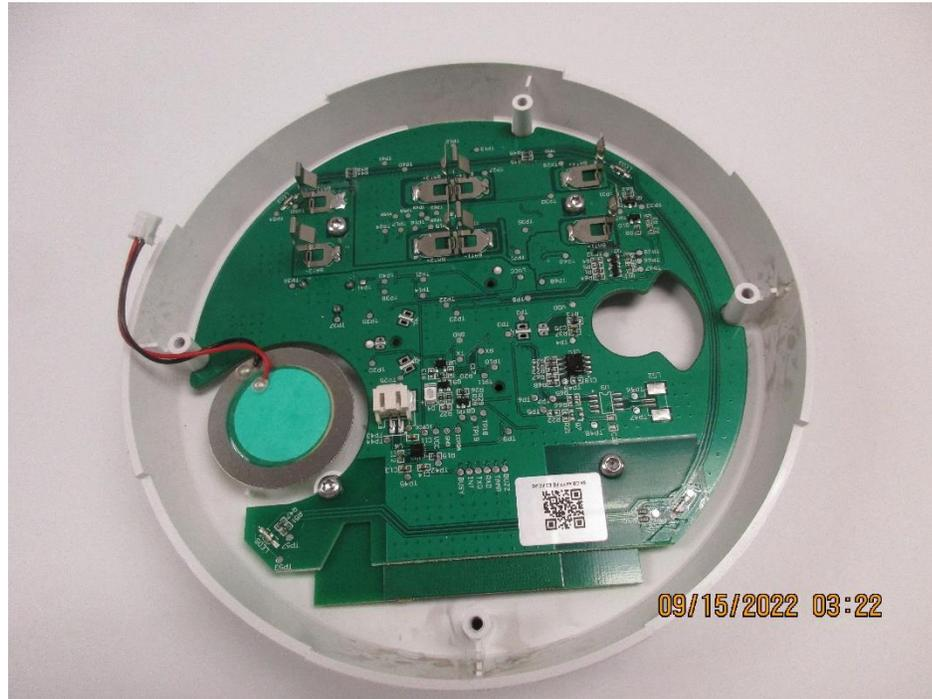
Figure 3 PCB without battery holder
