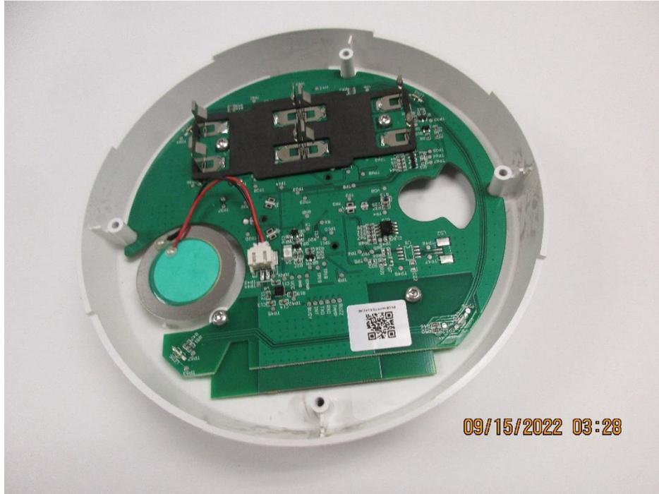
Figure 1 PCB with Battery holder]
