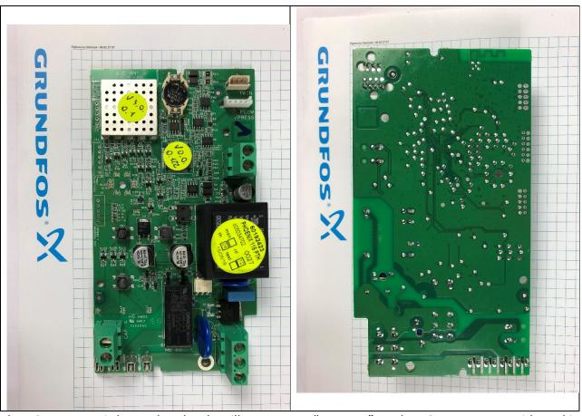
The PCB antenna is located under the silkscreen text "BLE ANT" on the PCB component side and is visible on the non-component side of the module PCB
