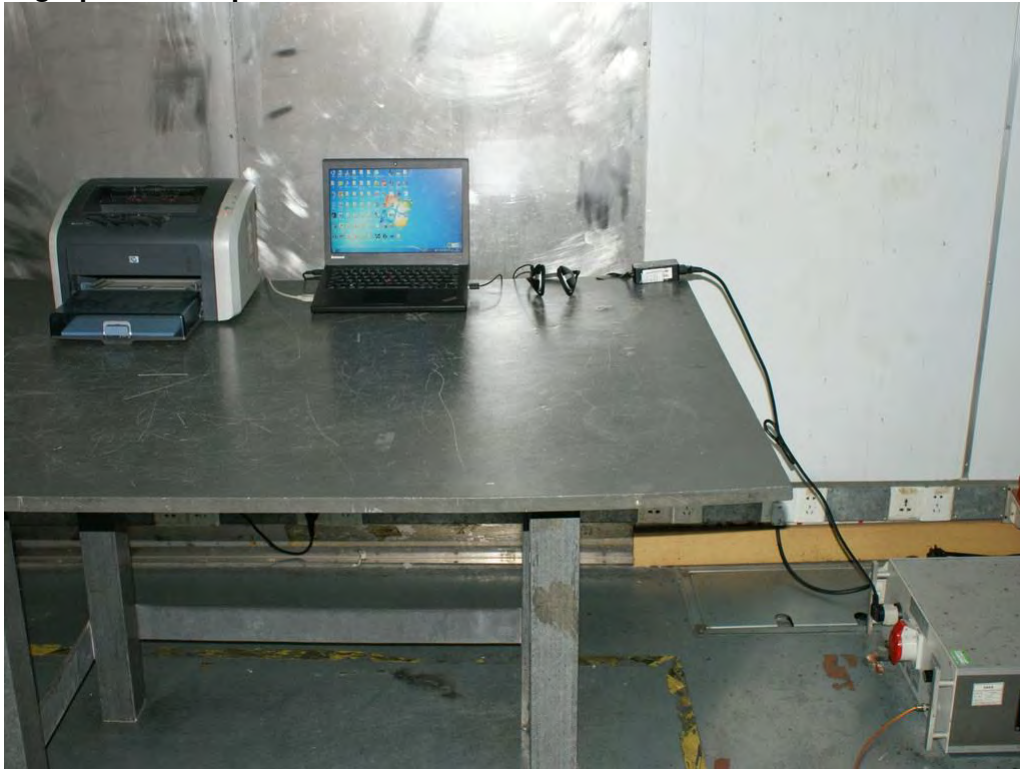
Photograph 2: Set-up for Spurious Emissions for below 30MHz
