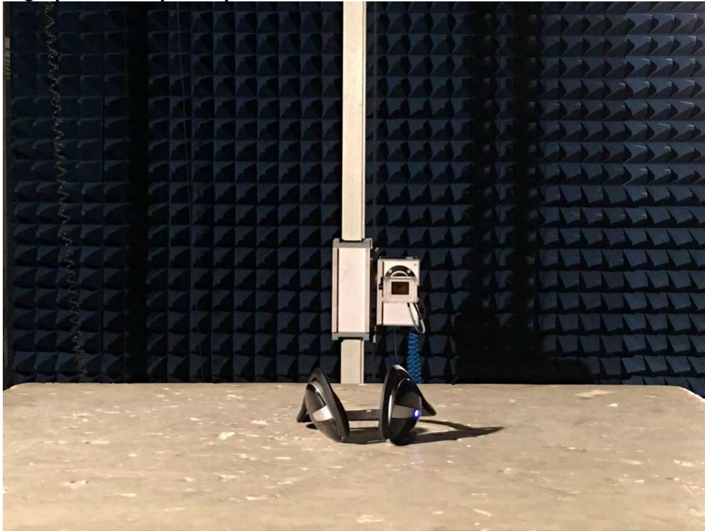
Photograph 5: Set-up for Spurious Emissions for 18 - 25GHz
