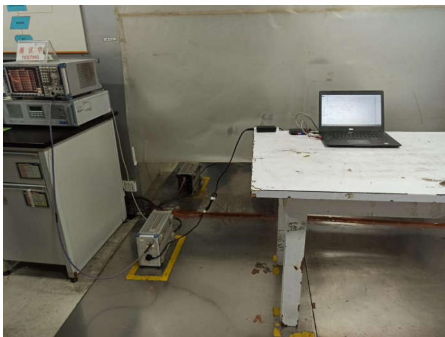
Conducted Emissions Test Setup
