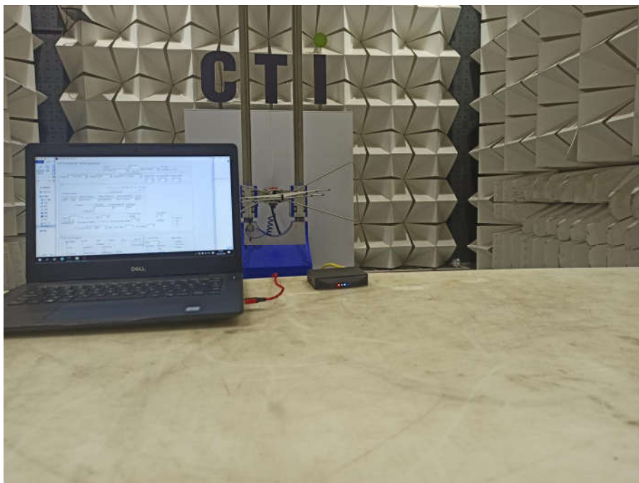
Radiated spurious emission Test Setup-2(Below 1GHz)
