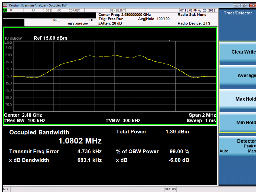
Plot 7-3. 6dB Bandwidth Plot (Bluetooth (LE) – Ch. 39)
