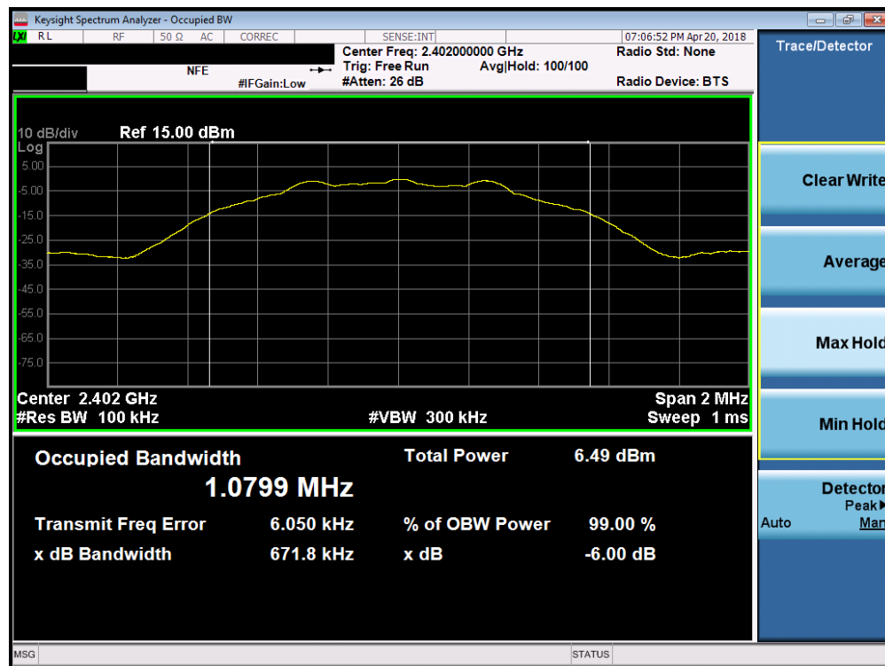
Plot 7-1. 6dB Bandwidth Plot (Bluetooth (LE) – Ch. 0)
