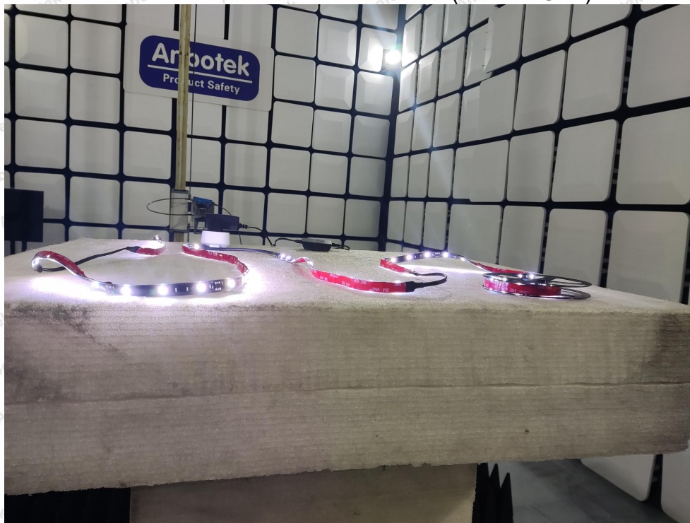
Photo of Radiation Emission Test (above 1GHz)
