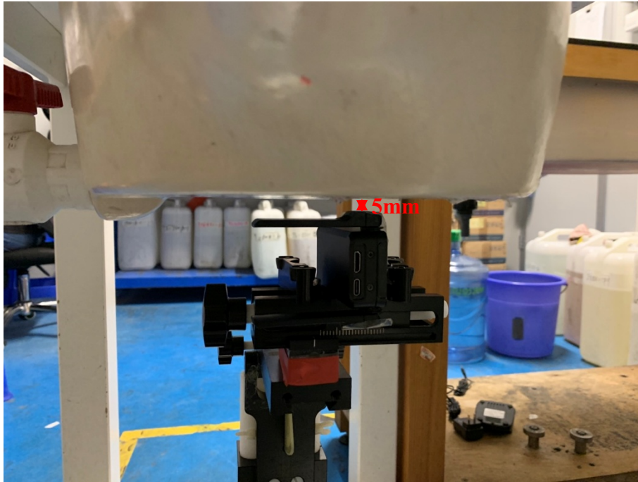
Front Side With Antenna Fold (Chain 1)Setup Photo(5mm)
