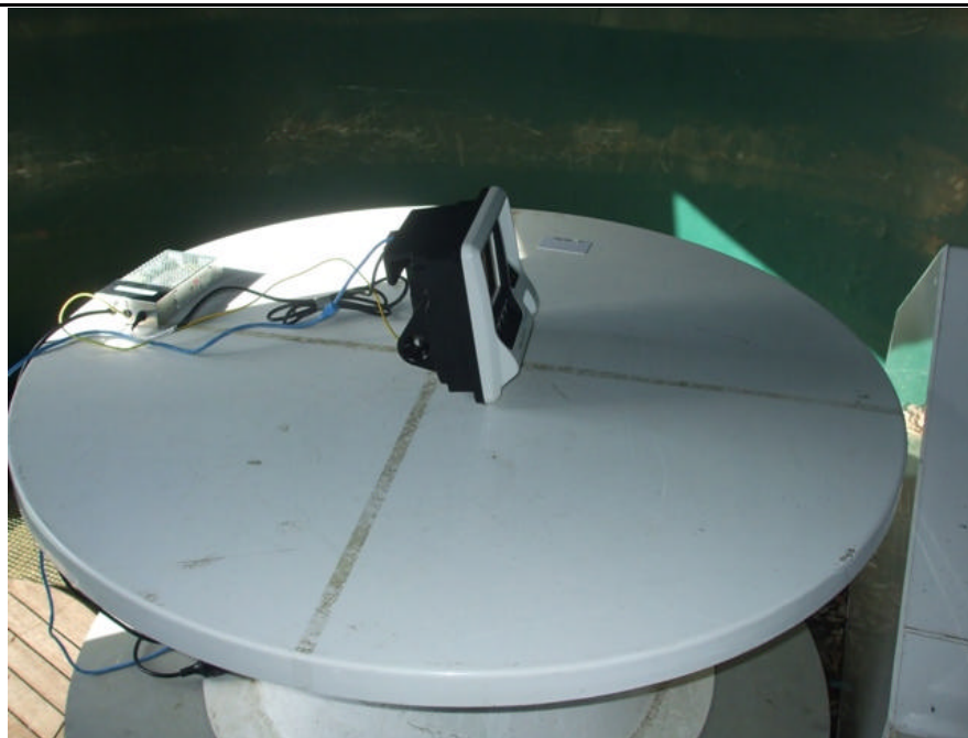
Conducted emissions test set up
