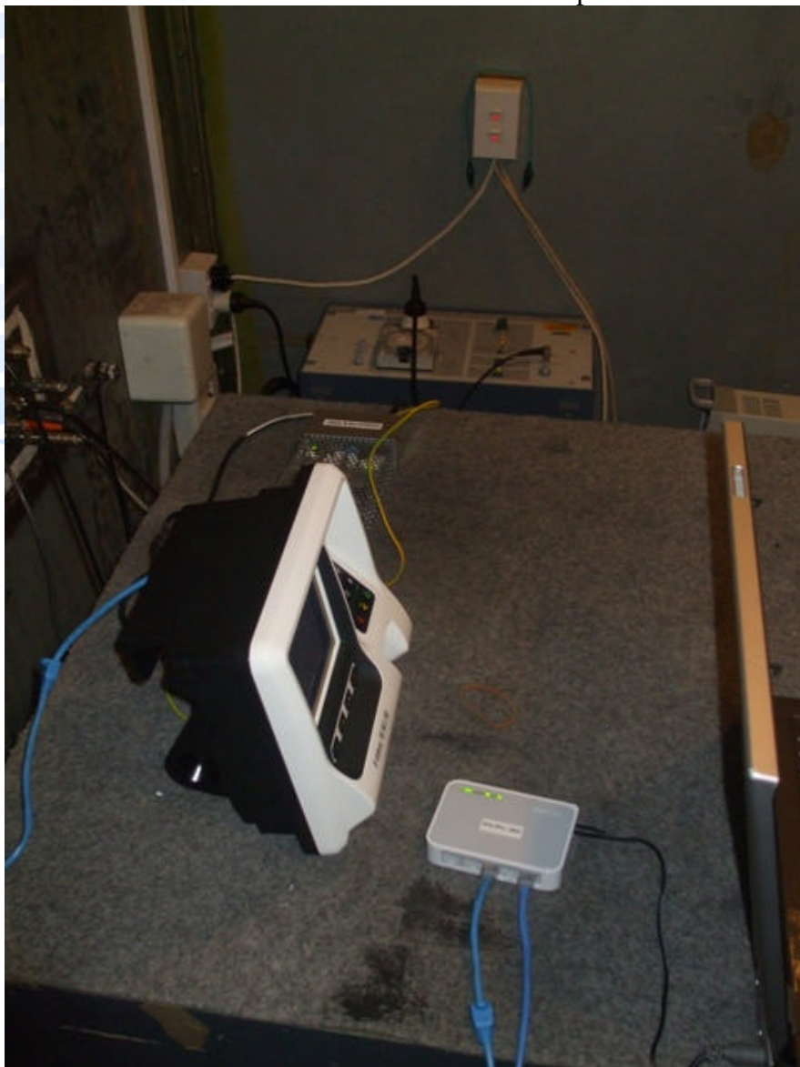
Conducted emissions test set up
