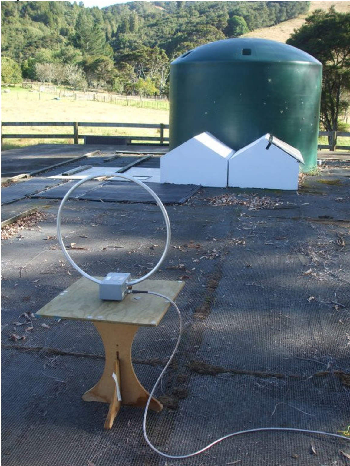
Loop antenna at 10 metres below 30 MHz
