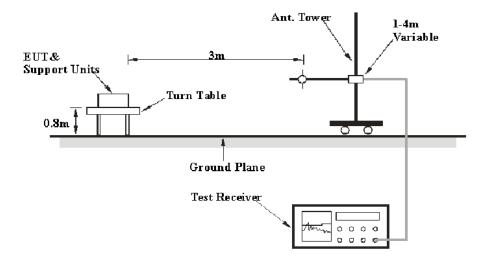
The radiated emission tests were performed in the 3 meters chamber test site, using the setup accordance with the ANSI C63.10-2013. The specification used was the FCC 15.209 and FCC 15.205 limits.
