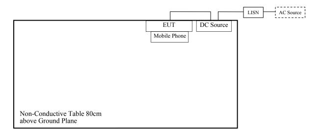
For Radiated Emissions (Below & Above 30MHz):
