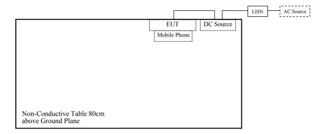
For Radiated Emissions (Below & Above 30MHz):
