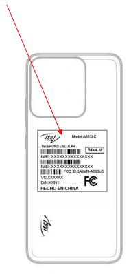
The label shown shall be permanently affixed at a conspicuous location on the device and be readily visible to the user at the time purchase (Labeling requirements per 2.925)
