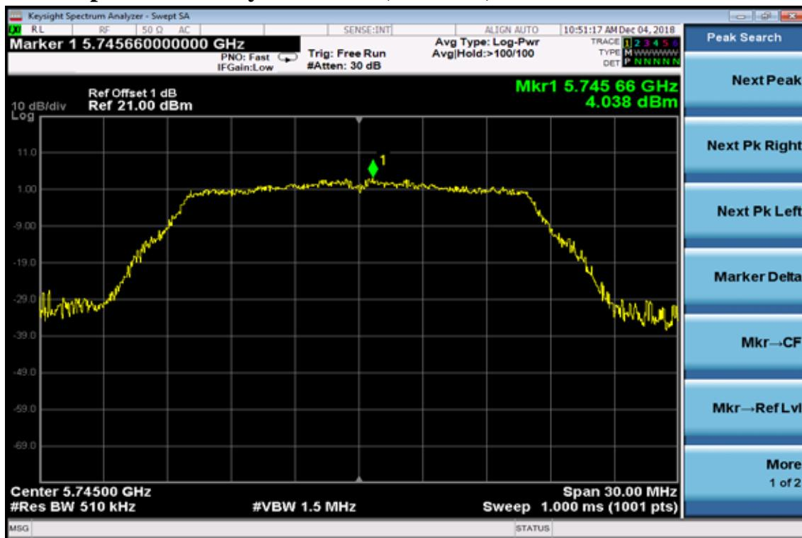
**Power Spectral Density Data Plot (CH Mid)**
