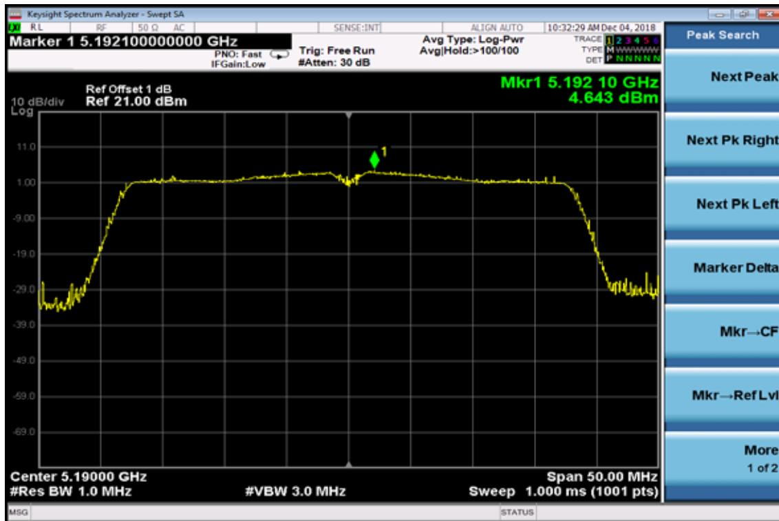
**Power Spectral Density Test Plot (CH-Mid)**
