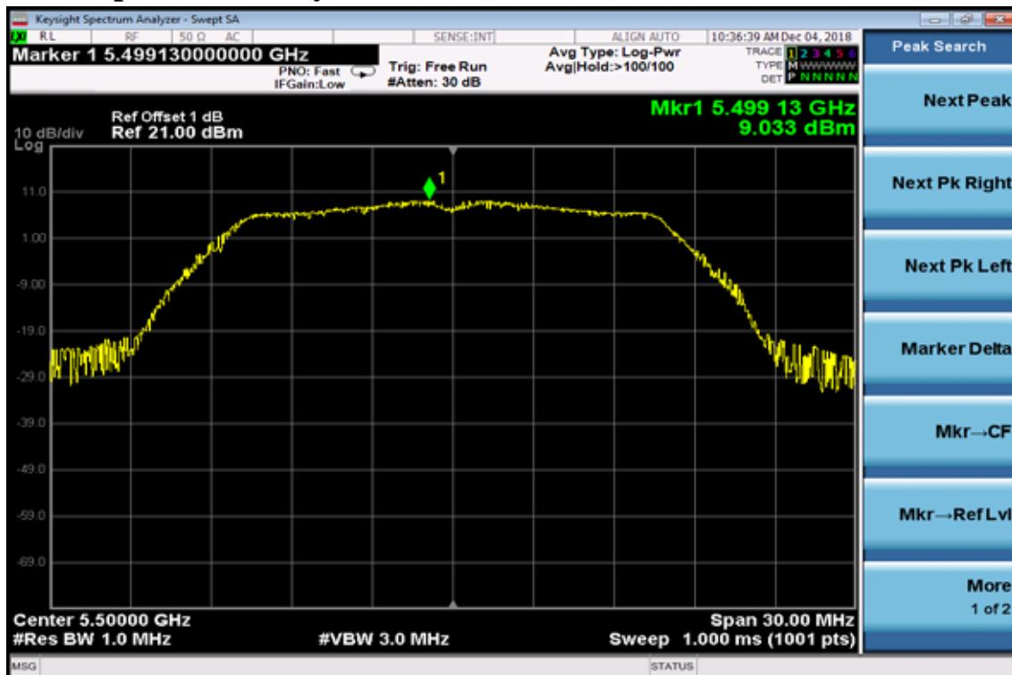
**Power Spectral Density Data Plot (CH Mid)**
