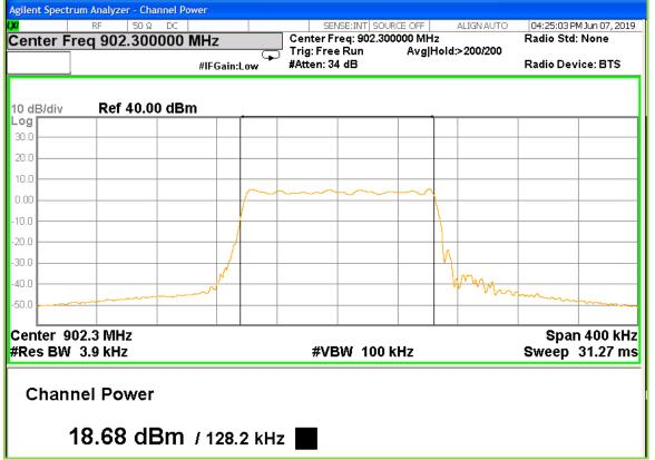
Screen Captures from the spectrum analyzer: 125 KHz MID Channel (Hybrid Mode)
