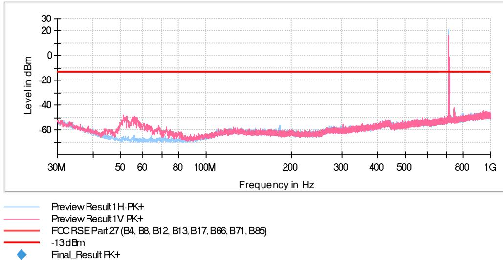
The peak above the limit is the LTE Cat-M1 Band 85 carrier frequency.
