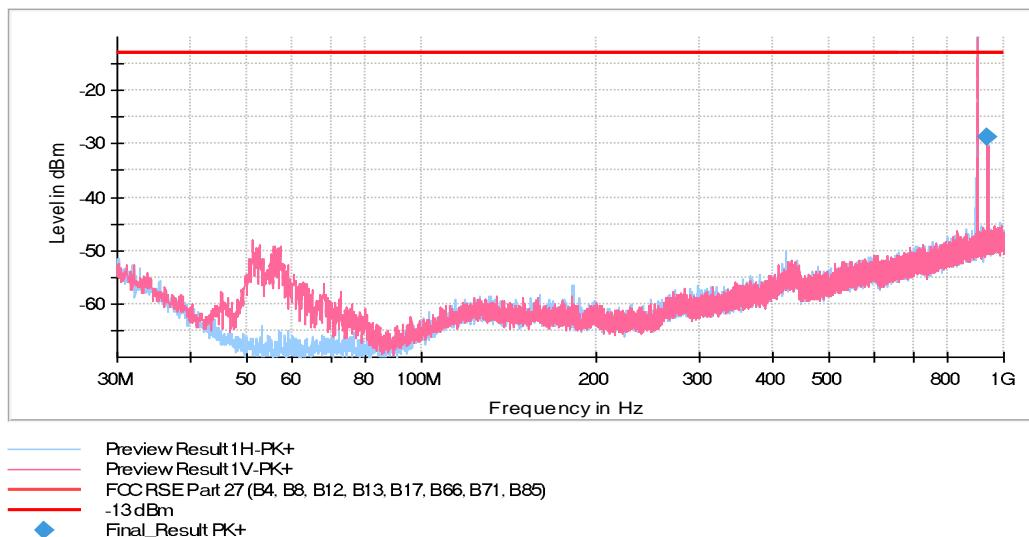
The peak above the limit is the LTE Cat-M1 Band 8 carrier frequency.
