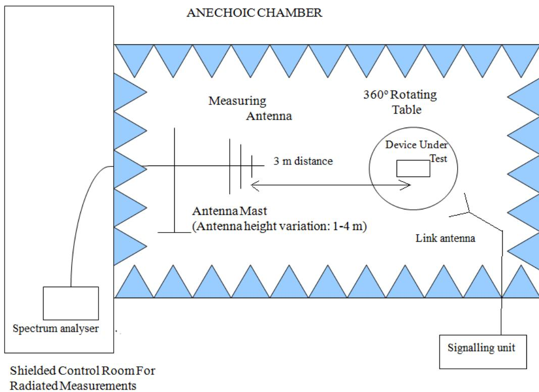
Radiated measurements setup from 1 GHz to 17 GHz:
