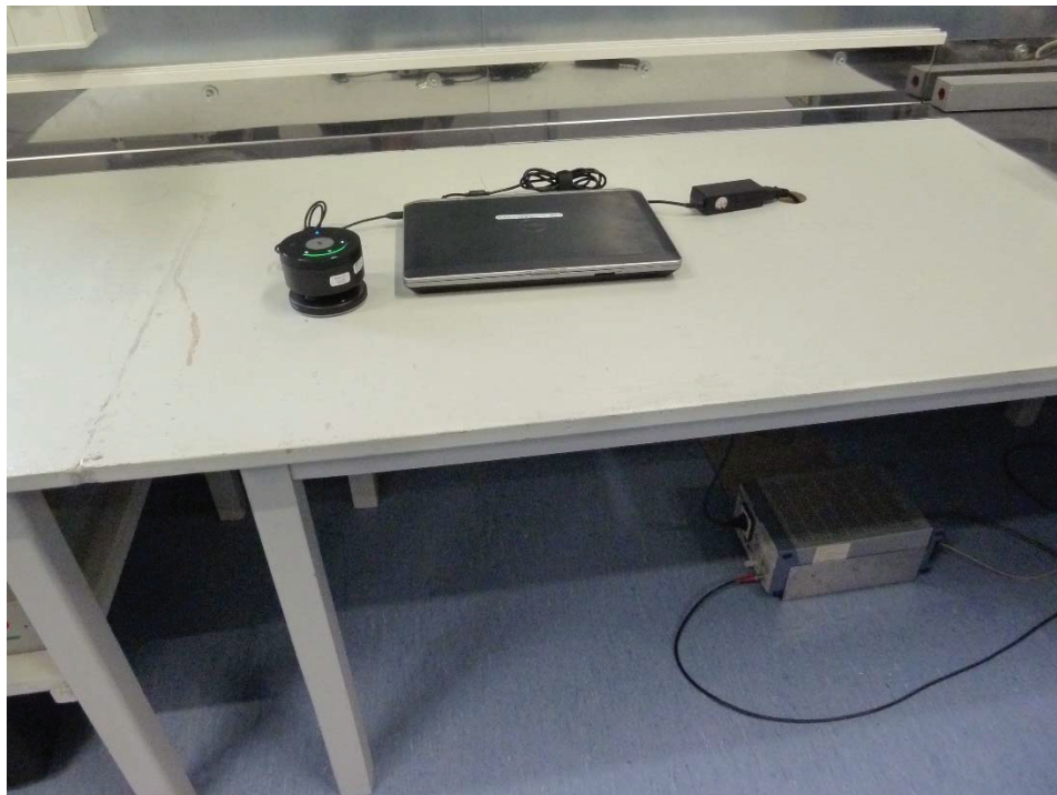
Photo 1: Power Line Conducted Emission Test
