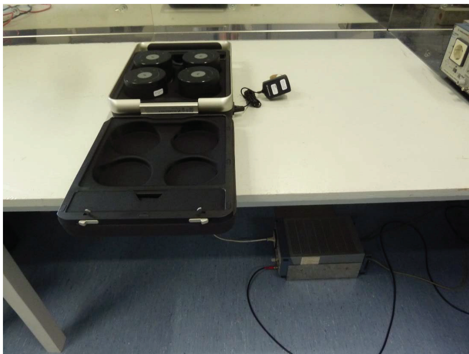
Photo 1: Power Line Conducted Emission Test
