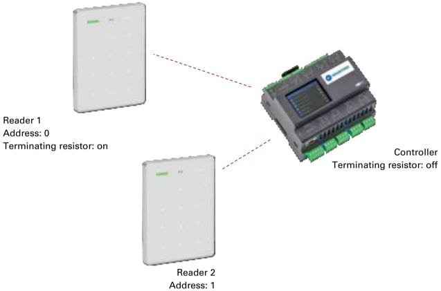
Terminating resistor: on
