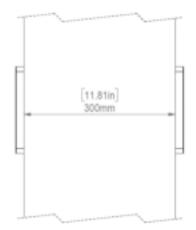
Fig. 2 - Example 1: installation of 2 readers next to each other
