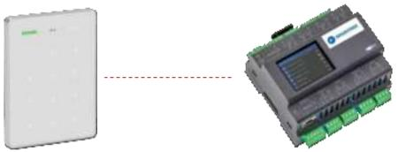
Reader Address: 0 Terminating resistor: on
