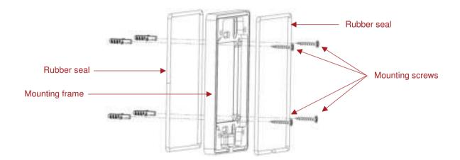
2. The mounting frame is equipped with a cable inlet on its bottom side, which also serves as a cable strain relief. Optionally, the cable inlet can be sealed with silicone.
