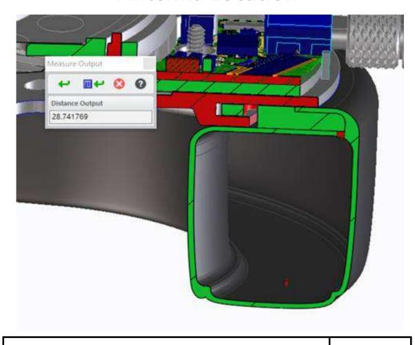
Separation Distance Between BT Antenna and Human (mm)
