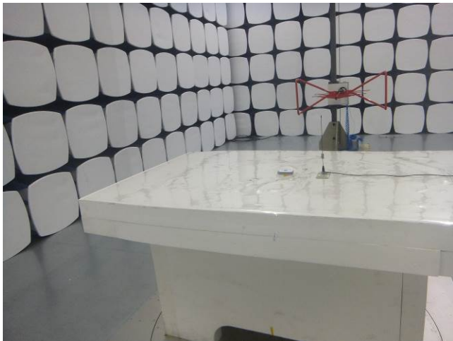
Radiated Spurious Emissions Test Setup Below 1GHz
