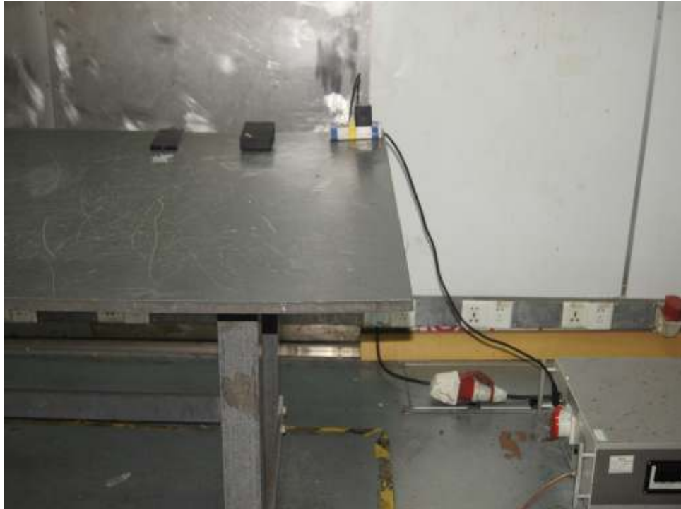
Photograph 7: Set-up for Conducted emissions
