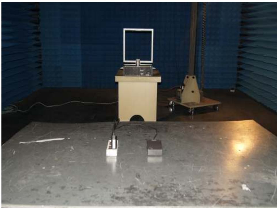
Photograph 2: Set-up for Spurious Emissions (30MHz-1GHz)
