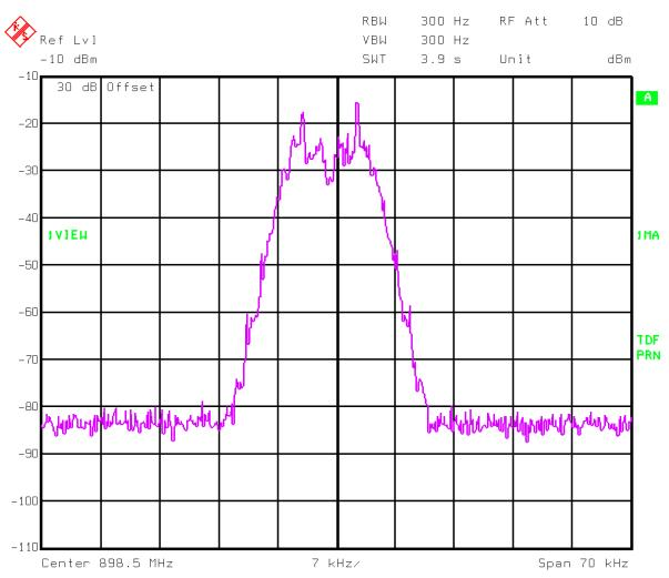
Title: occupied bandwidth 2 fsk input uplink Comment A: occupied bandwidth uplink input 2 fsk
