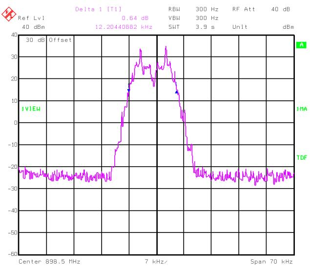
Title: occupied bandwidth 2 fsk output uplink Comment A: occupied bandwidth uplink output 2 fsk
