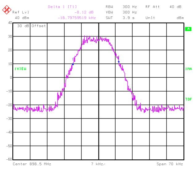
Title: occupied bandwidth 4 fsk output uplink Comment A: occupied bandwidth uplink output 4 fsk
