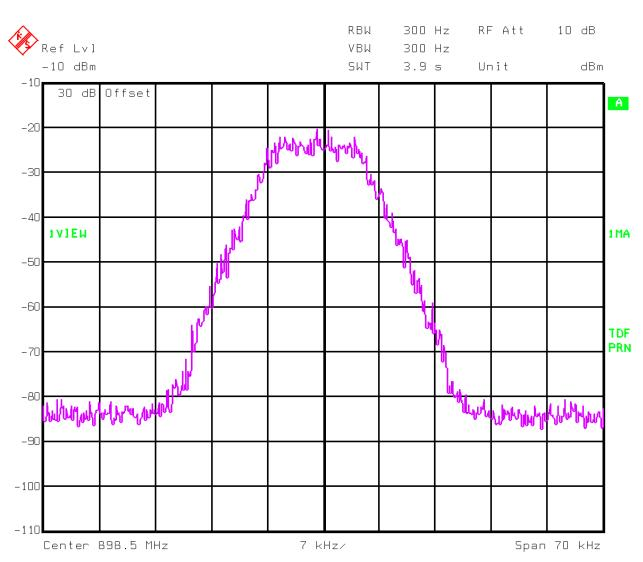
Title: occupied bandwidth 4 fsk input uplink Comment A: occupied bandwidth uplink input 4 fsk
