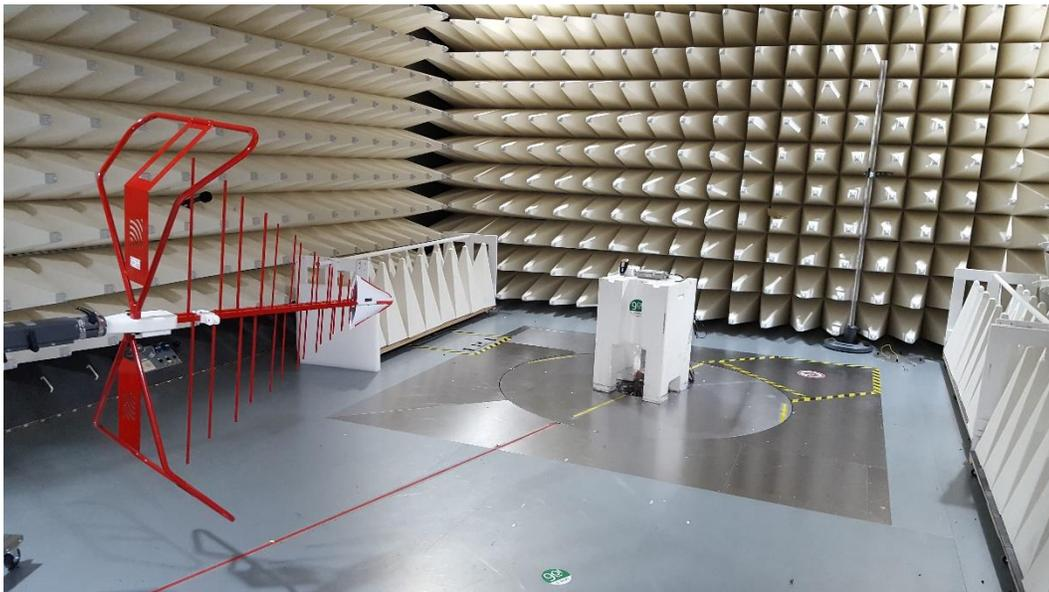
Figure B6. Radiated emission Setup 2
