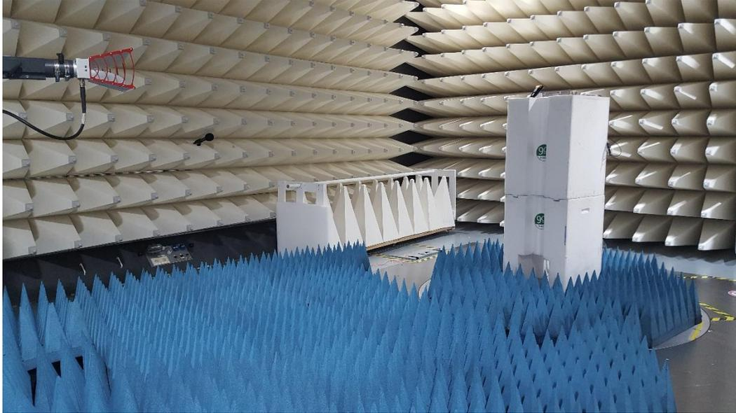
**Figure B7.** Radiated emission Setup 2
