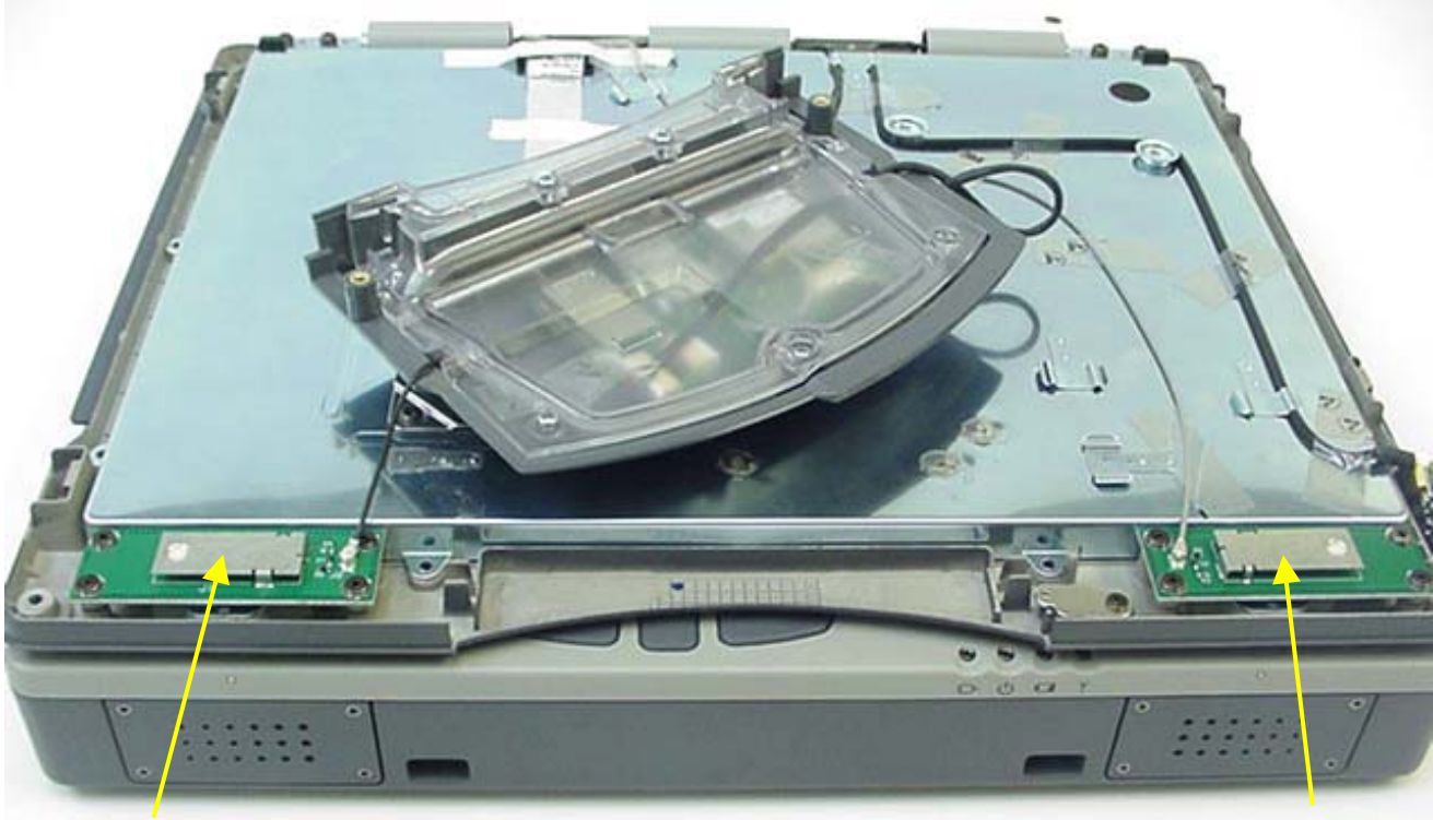
Bluetooth Surface-Mount Antenna (Upper Rear Left Side of LCD Display)
