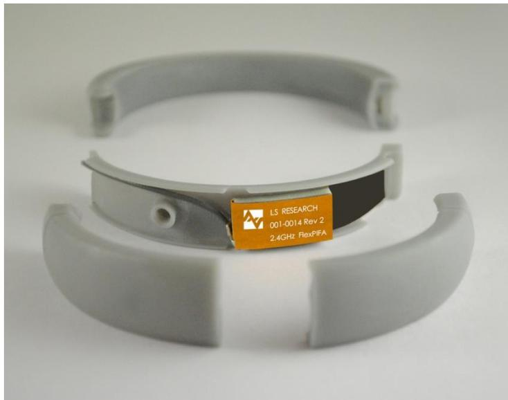
**Figure 30 FlexPIFA Integrated into Bracelet**
