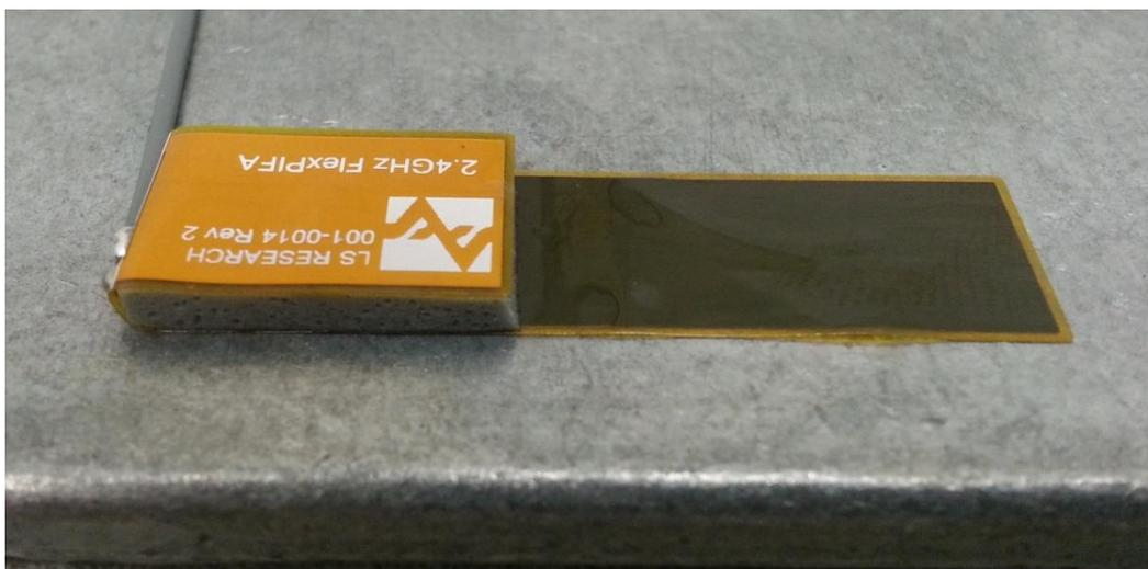
**Figure 27 FlexPIFA Mounted on Metal**
