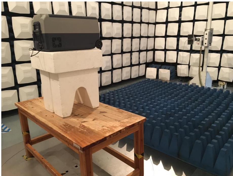
Test Setup For Radiated Emission (Above 1GHz)
