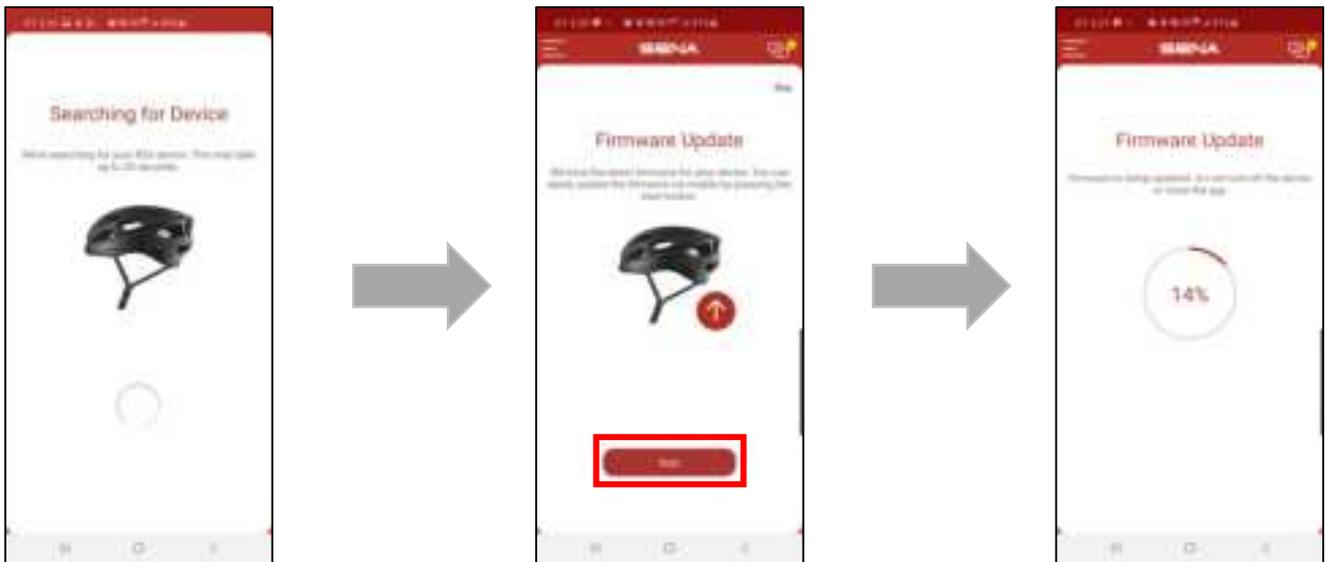
3.1.3 When the firmware update is complete, the [Firmware Update Complete] screen automatically moves to the [Name Your Device] screen.
