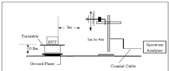
3. Radiated Emission Test-Up Frequency Above 1GHz
