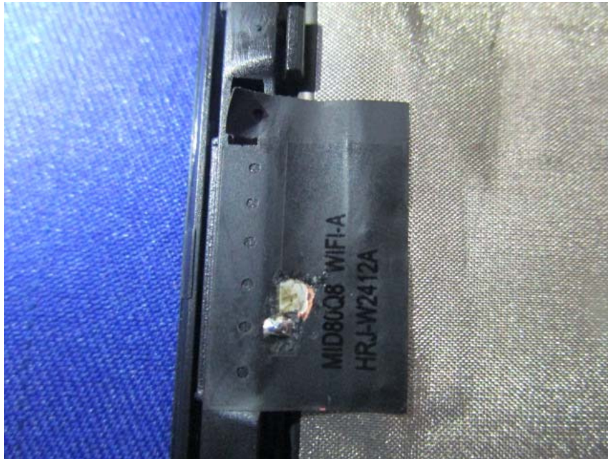
EUT –Wifi &BT Antenna View
