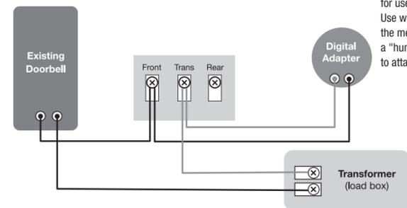
The **Digital Adapter** is required for use with a Digital Doorbell. Use with a mechanical chime if the mechanical chime develops a "hum". The sticker can be used to attach adapter to the chime.
