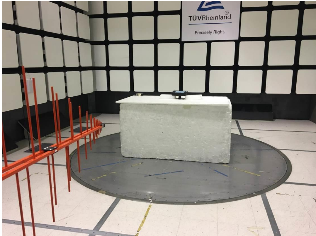
Figure 2: Test Setup for Radiated Emissions 30 MHz to 1000 MHz - Front
