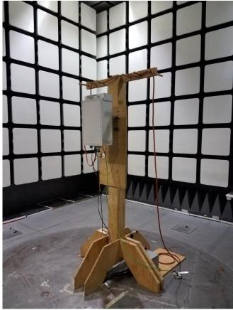
Radiated Setup for Channel Power, Occupied Bandwidth, Edge of band and Modulation.
