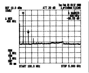
The plot overleaf shows the spectrum for the 121.5MHz transmission. It can be clearly seen that the only spurious are harmonics of 121.5MHz, which are more than 39dB below the wanted signal. These are of course significantly attenuated by the antenna characteristics.
