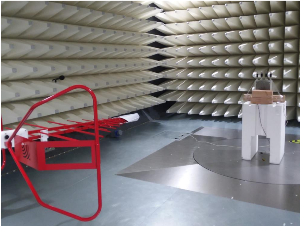
Figure B3: Low Range Radiated Emission test setup Using Biconical log antenna
