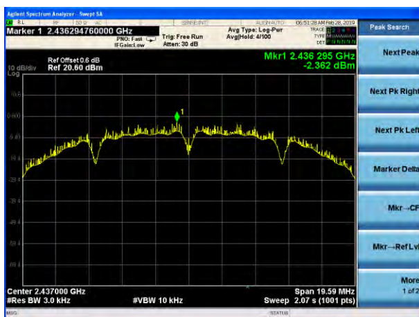
(802.11b) PSD plot on channel 6
