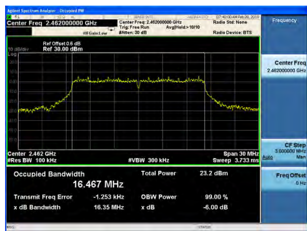
(802.11g) 6dB Bandwidth plot on channel 11
