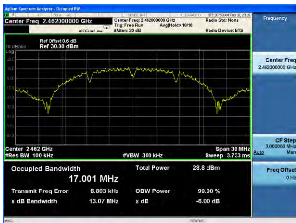
(802.11b) 6dB Bandwidth plot on channel 11
