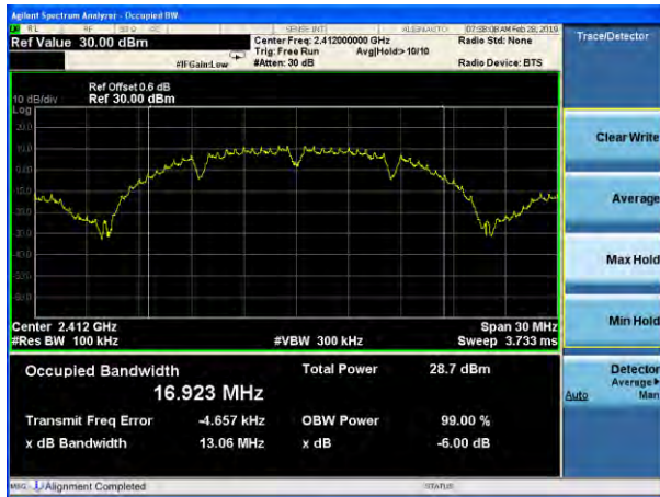
(802.11b) 6dB Bandwidth plot on channel 6
