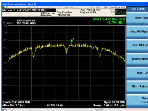
(802.11b) PSD plot on channel 6
