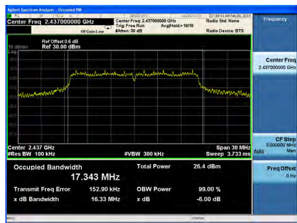
(802.11g) 6dB Bandwidth plot on channel 6
