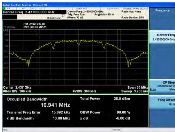
(802.11b) 6dB Bandwidth plot on channel 6
