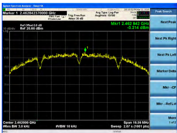
(802.11b) PSD plot on channel 11
