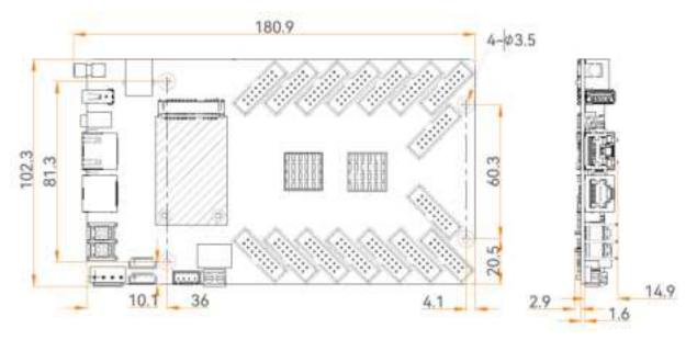
Tolerance: ±0.3 Unit: mm
