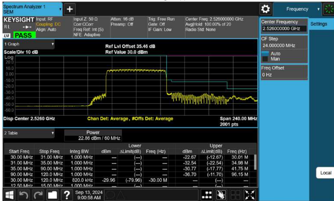
NR41_60 M_Channel Edge_Upper_Low_BPSK_FullRB
