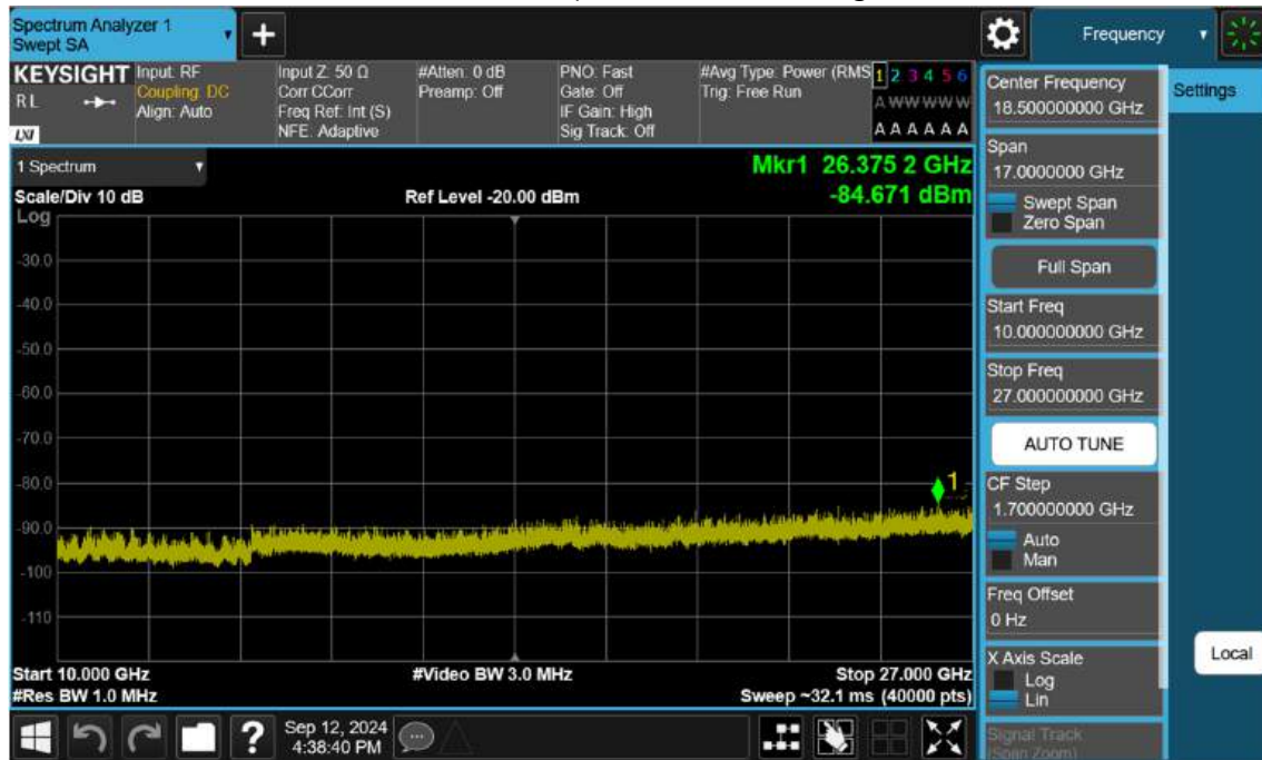
NR41_30 M_Conducted Spurious(Above10 G)_High_BPSK_1RB
