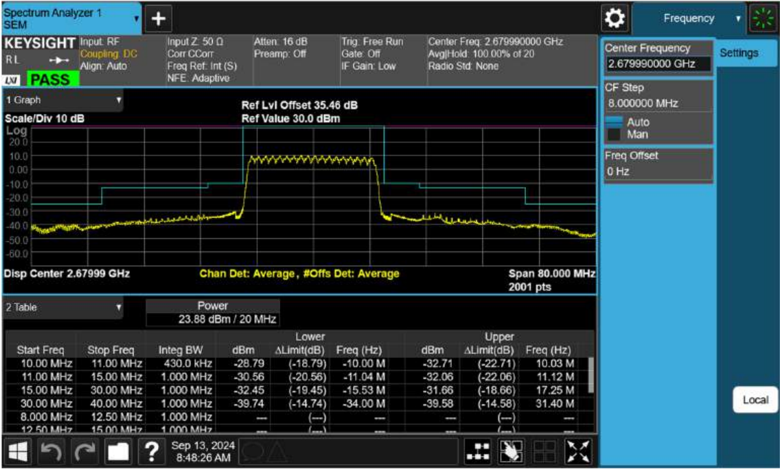
NR41_20 M_Channel Edge_High_BPSK_FullRB
