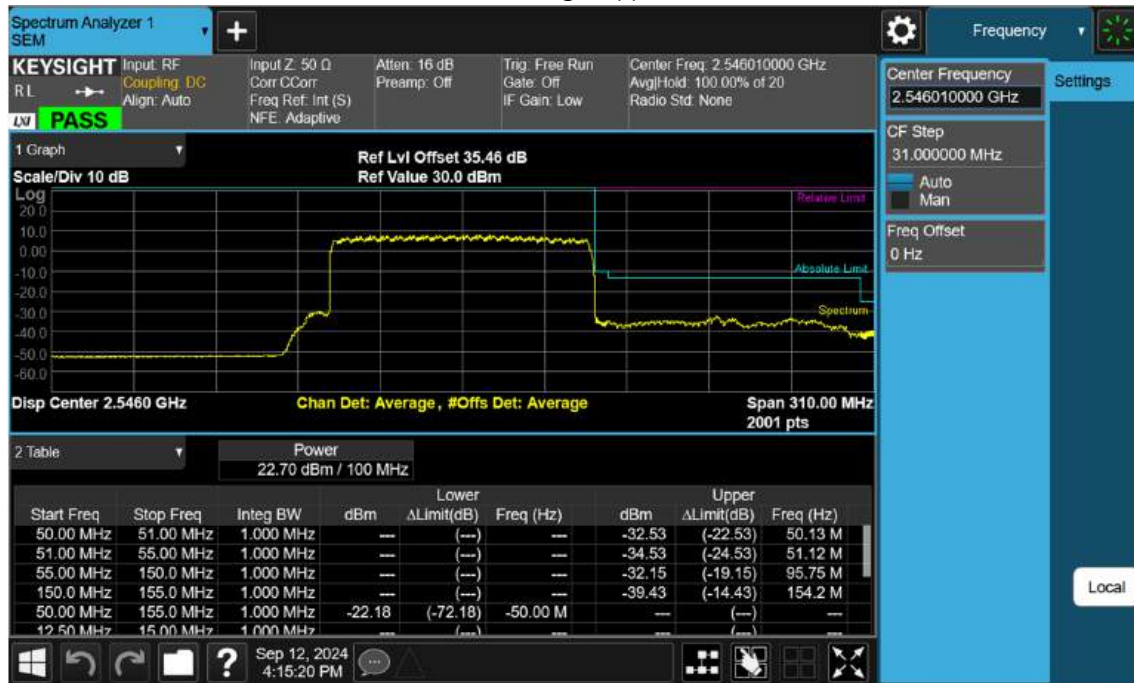
NR41_100 M_Channel Edge_Upper_Low_BPSK_FullRB
