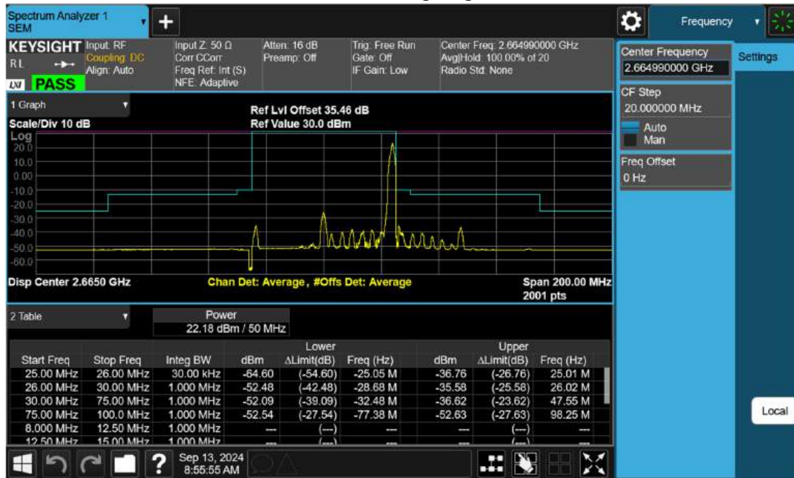
NR41_50 M_Channel Edge_High_BPSK_1RB
