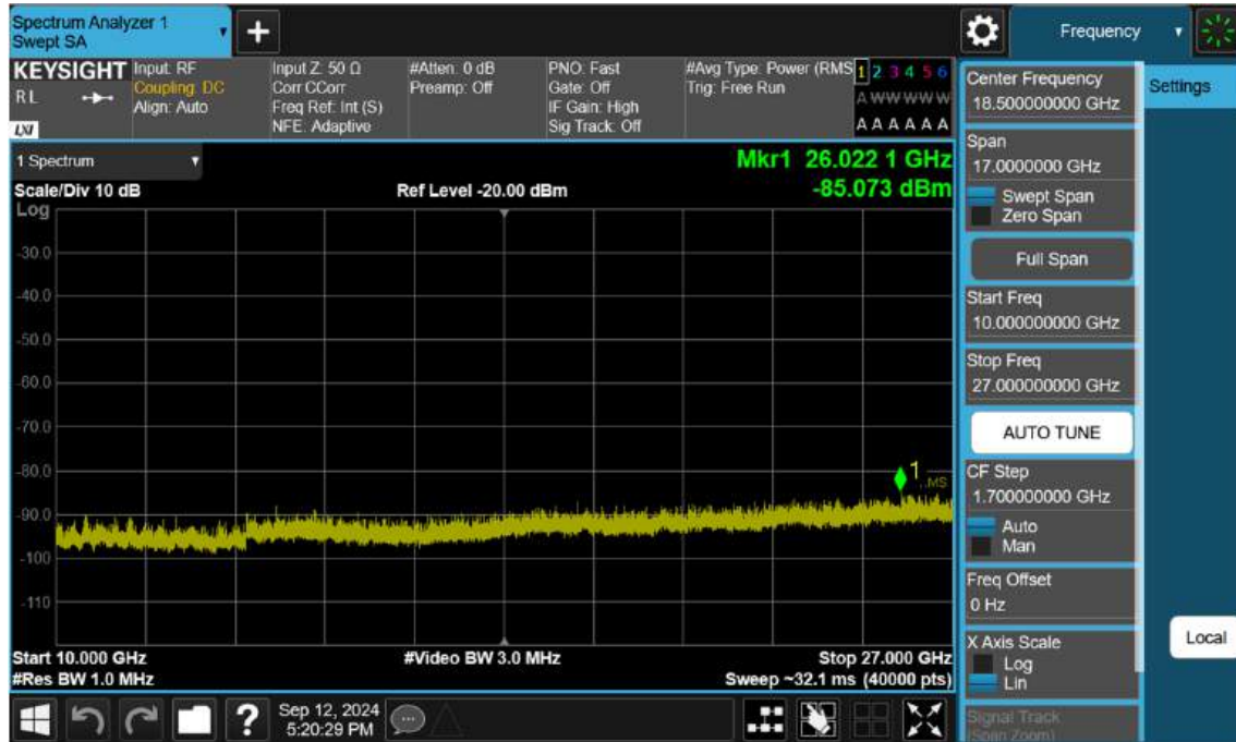
NR41_100 M_Conducted Spurious(Above10 G)_Low_BPSK_1RB
