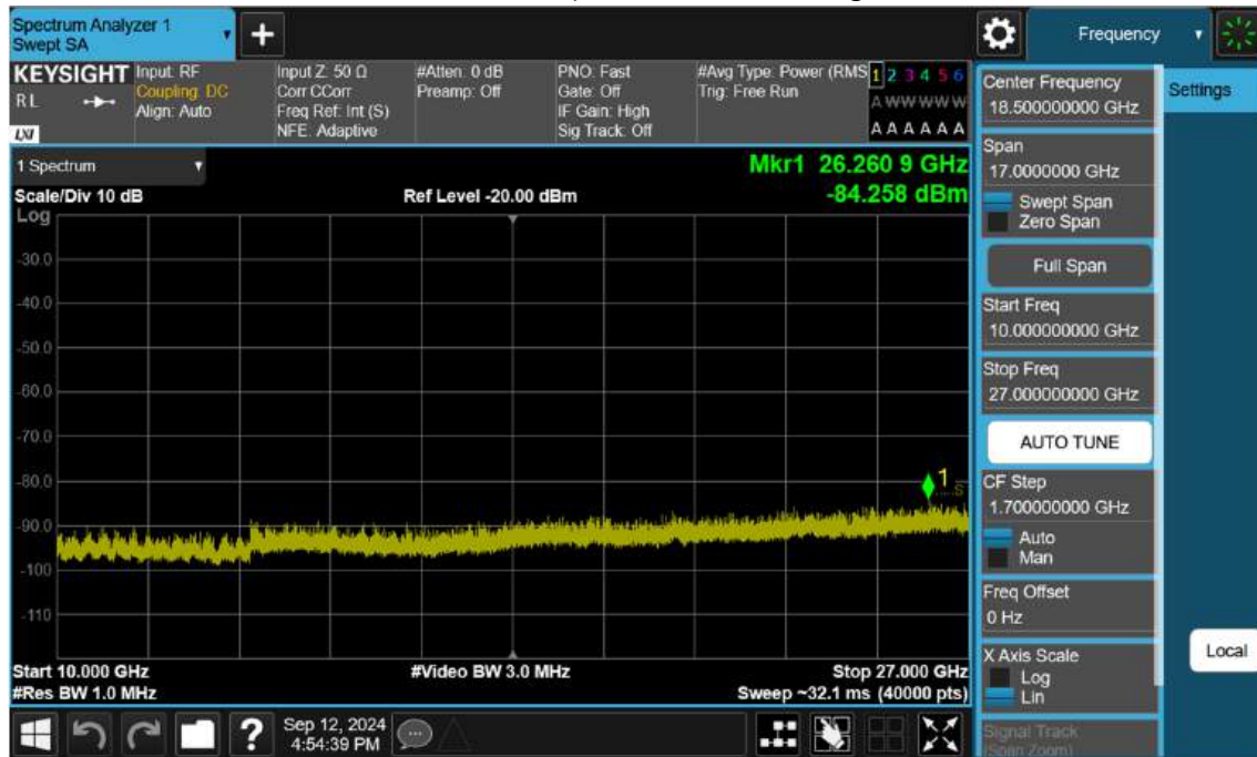
NR41_50 M_Conducted Spurious(Above10 G)_High_BPSK_1RB
