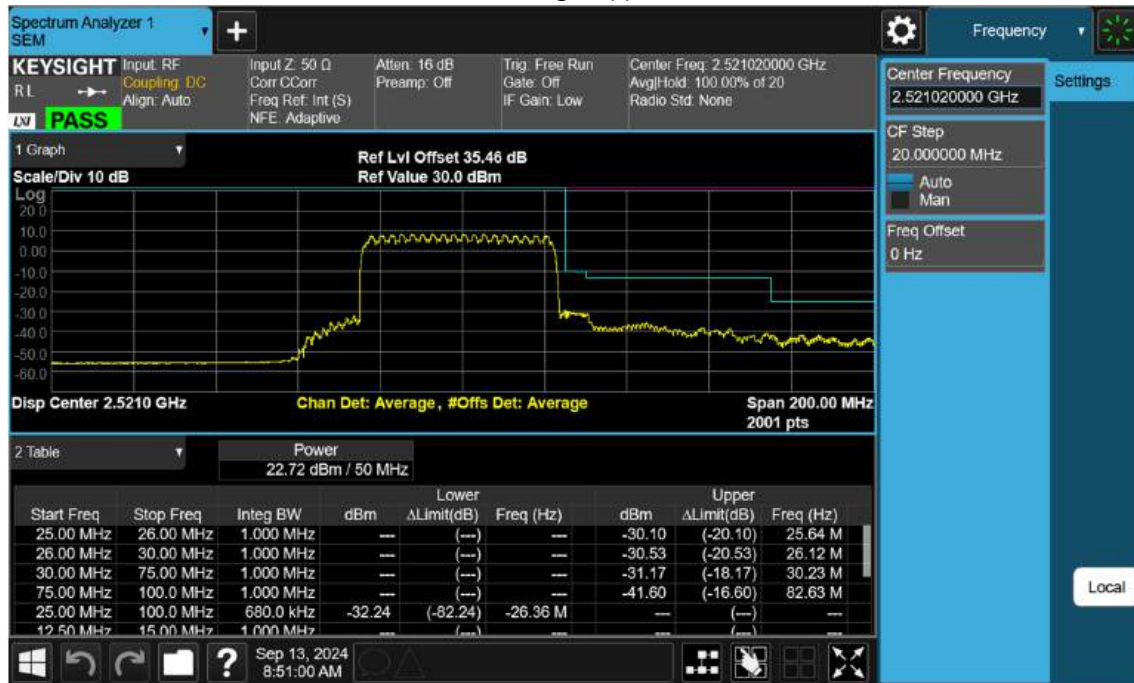
NR41_50 M_Channel Edge_Upper_Low_BPSK_FullRB
