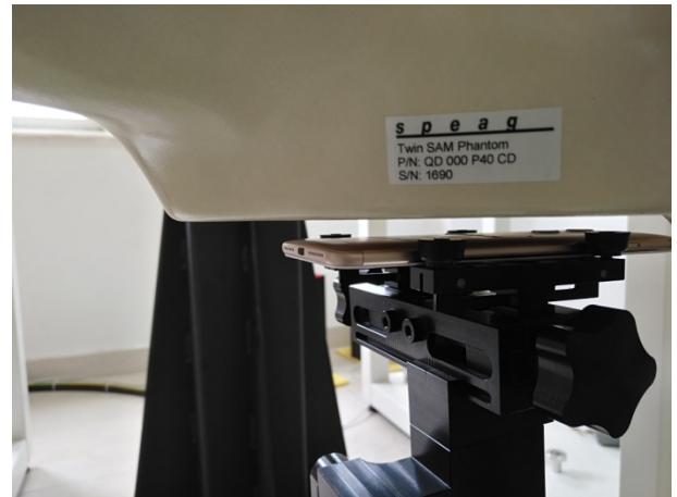
Body-worn Rear Side (10mm)
