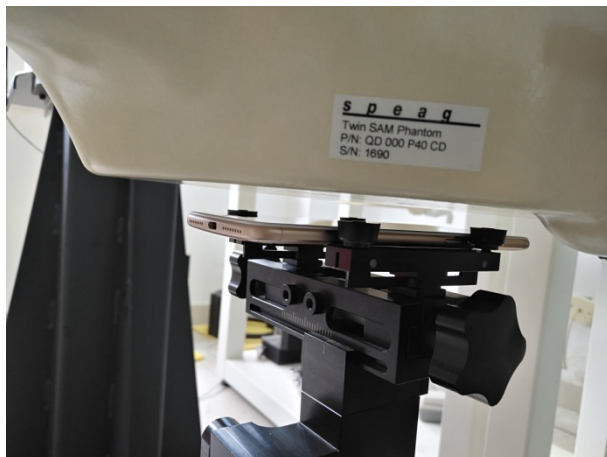
Hotspot mode - Front Side (10mm)
