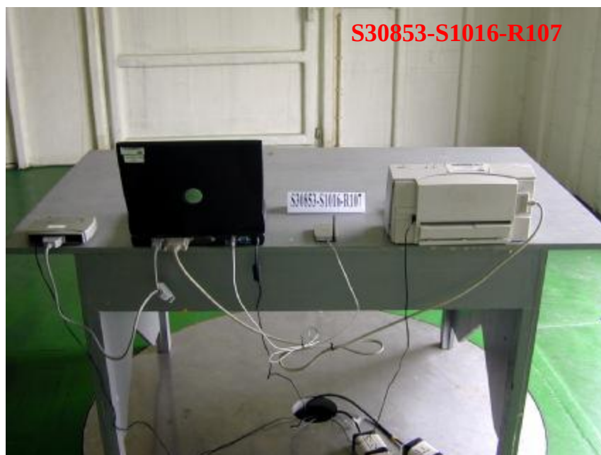
Photo 3: Radiated Emission Test Set-up
