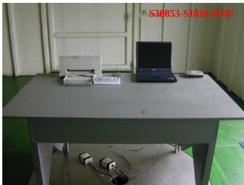
Photo 2: Radiated Emission Test Set-up
