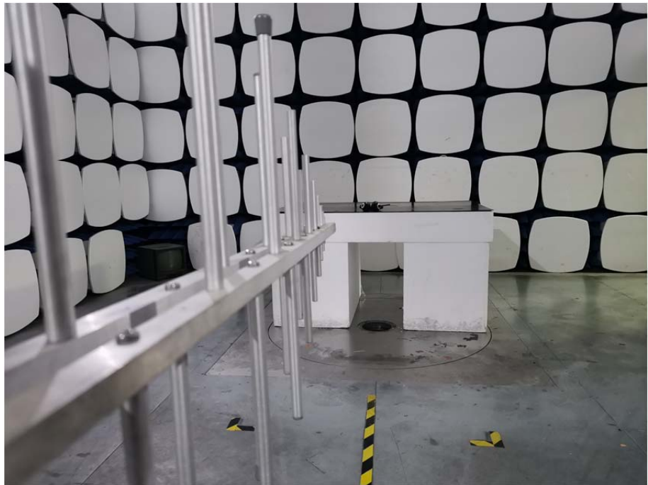
Radiation Emission Test Setup (30MHz to 1GHz)
