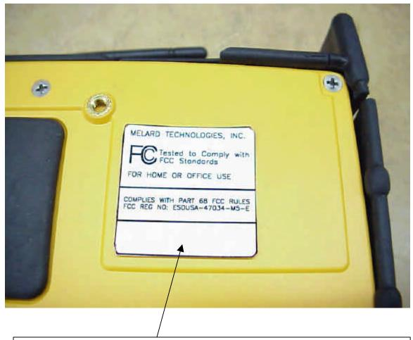
Insert radio modem FCC ID labels in this area.
