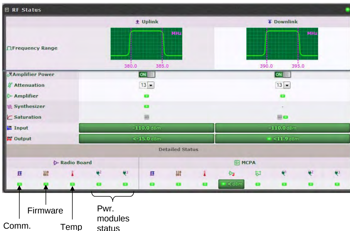
Figure 7-3: BSF-3604 Repeater Status
