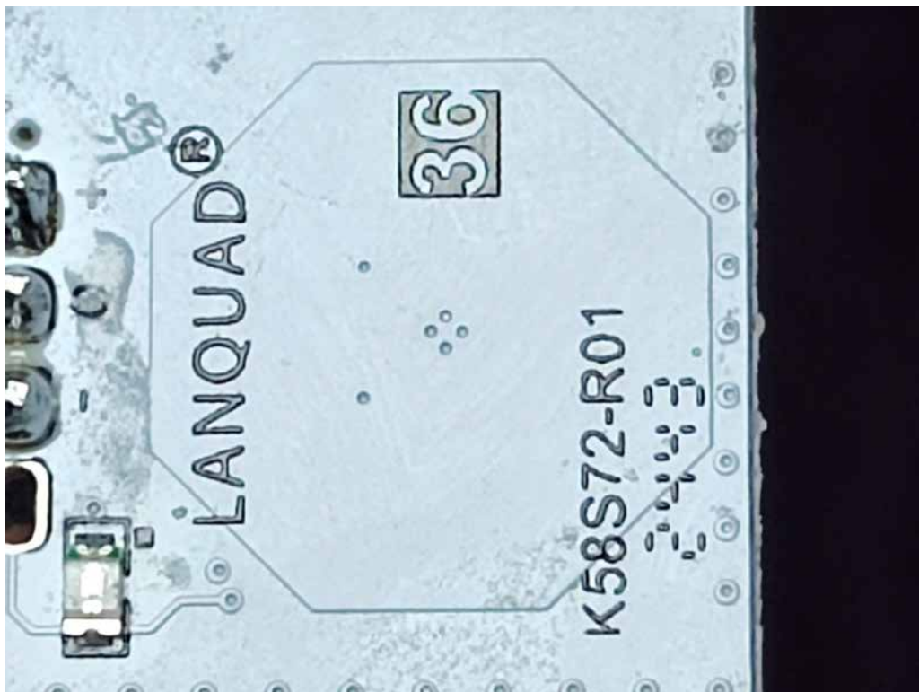
FIGURE 14 LED LAMP (G117P38MO6C) ANTENNA ON CONTROL BOARD
