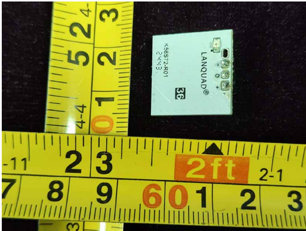
FIGURE 14 LED LAMP (G117P38MO6C) ANTENNA ON CONTROL BOARD
