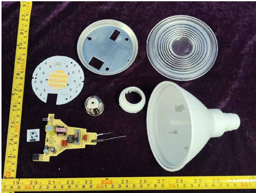
FIGURE 8 LED LAMP (G117P38MO6C) MAINBOARD FRONT
