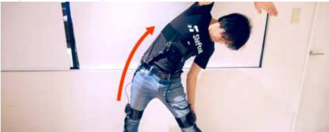
5. Make sure again that the straps are longer than the connecting cable.
