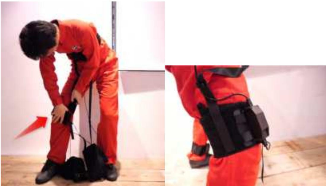
3. Attach the "Straps for below the knee" to your body. Wrap it around the area between your knees and ankles. As with the above the knee, if the sensor is misaligned, the tracking will also be misaligned, so make sure you wrap it tightly and firmly.
