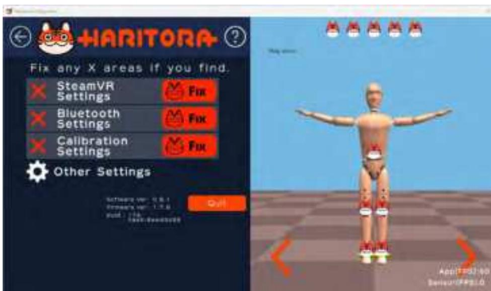
On the right is a dummy representing the whole body motion calculated by Haritora Configurator. This dummy's posture moves the avatar on the VR application.
