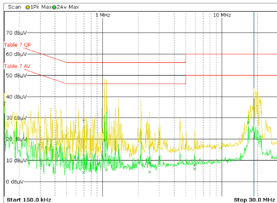
Line N Conducted Emission Graph
