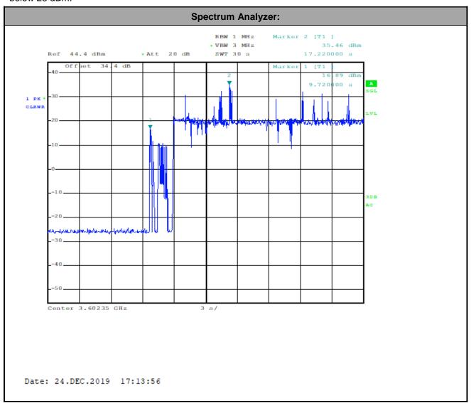
Note: The Ref Offset 34.44 dB includes the antenna gain 19.44 dBi and cable path loss 15 dB.
